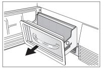
**5.** Remove fluff from the fluff filter on the floor of the base with a damp hand.
